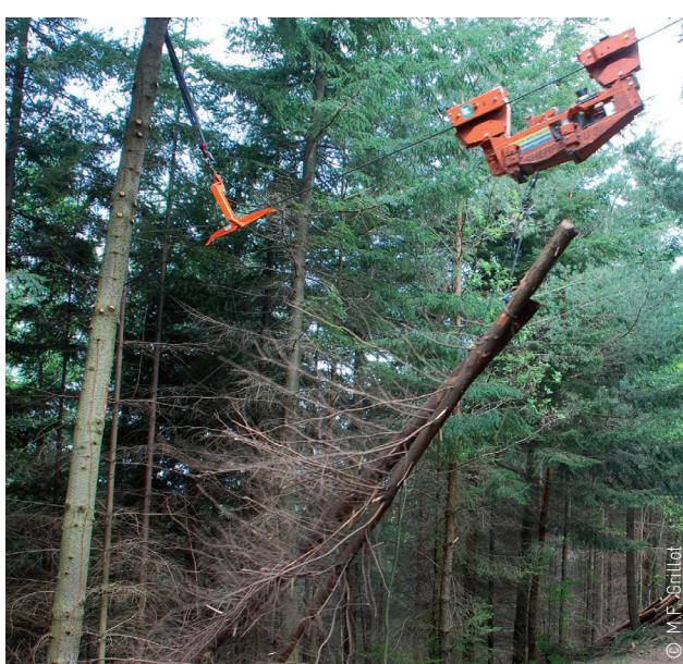
Fig. 3: Cable logging, is now in general use in catchment protection areas in Masevaux (68).
